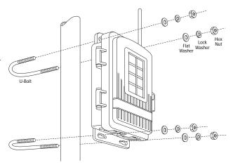
4. Place the second U-bolt around the pole and through the two holes at the bottom of the shelter. Put a flat washer, a lock washer, and a hex nut on each bolt end, and tighten the hex nuts.
