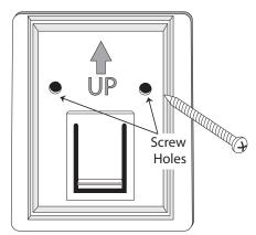
3. Slide the sensor housing down onto the bracket. It will click into place.
