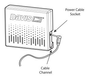
Tip: There is a cable channel in which to run the cable.
