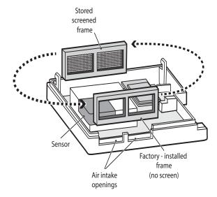
Put the unscreened frame into the empty storage slot and close the sensor housing.
