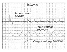
Fig. 5-2 Input inrush current, zoom into first peak 230Vac input, 24V 5A output, 25°C ambient
