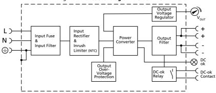
Fig. 11-2 Functional diagram PIC120.242C
