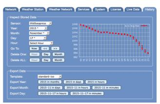
**Sharing -** Meteobridge PRO allows to export stored weather data in a CSV like notation. Which data to export and for what period in time is user-defined. This allows you to export data for various follow-on processes. Meteobridge PRO makes data exports accessible by providing a samba share (windows network folder) that every PC in your LAN can easily mount as a network folder.
